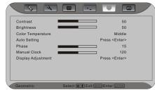
Display Adjustment- Press the ENTER button to confirm for sub-selectiion as shown in the OSD below then press button to adjust the position of display.
